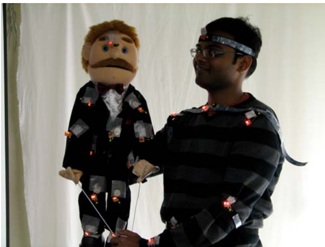
Figure 1. Player controlling a hand puppet. Both the player and puppet are tracked using LEDs.
