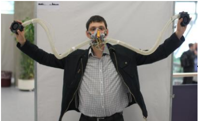
Figure 3 Stereo Olfacticon. Inspired by directional olfactory abilities of Luna Moths, twin fans temporally modulate spatially separated intakes, granting users a new sense to explore complex environments.
