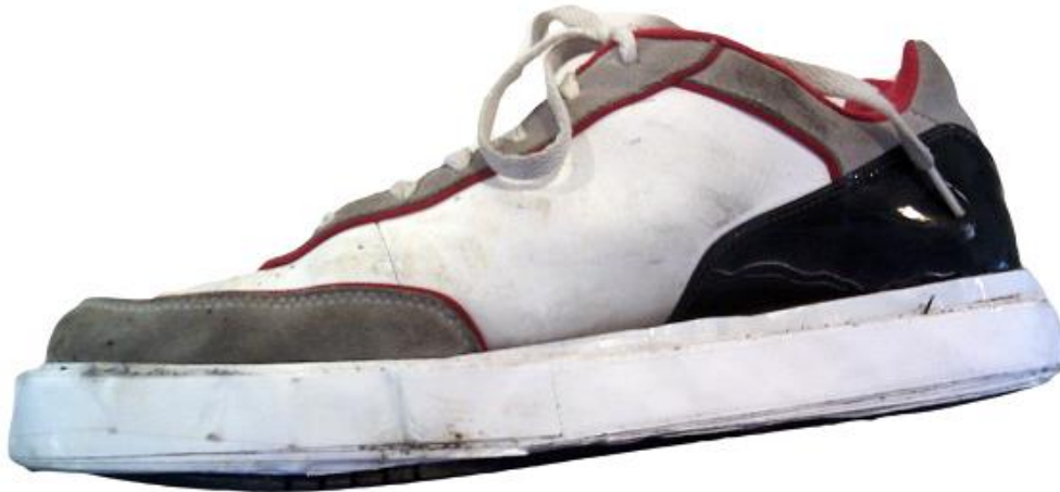
Figure 7. Prototype “Fresh Kick” constructed from bilayers of hard cellulose outer-tape and resilient, thick duct-tape inner-tape.
