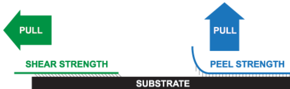
Figure 10. Diagram explaining the dimensional reduction of peeling layers of a tape-like substance. ( http://www.agpa.uakron.edu/p16/lesson-print.php?id=how_sticky_is_your_tape )
